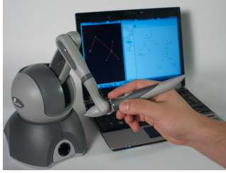
Figure 3: Interacting with the spatial haptic view using the stylus of a PHANTOM Omni haptic device.
