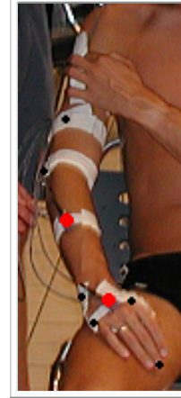
Figure 2: Sensor setup used to measure the pressure data at hand palm, hand back, elbow and shoulder.
